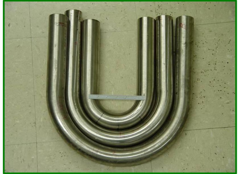
Cold-bent tubes are being creep tested to provide guidance for determining fabrication rules for Ni-base alloys
