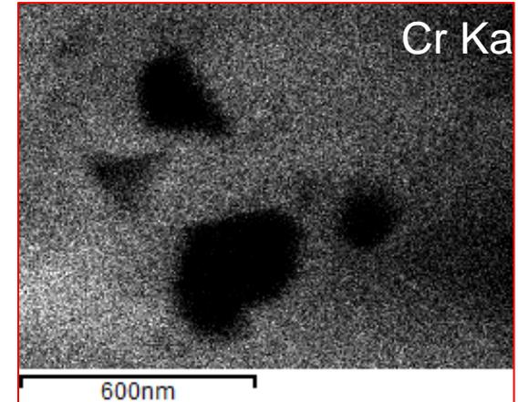
Small nano-scale Y-only particles were not identified through the EDX mapping. But coarser (100-200nm) Y-Si-O rich areas are seen
