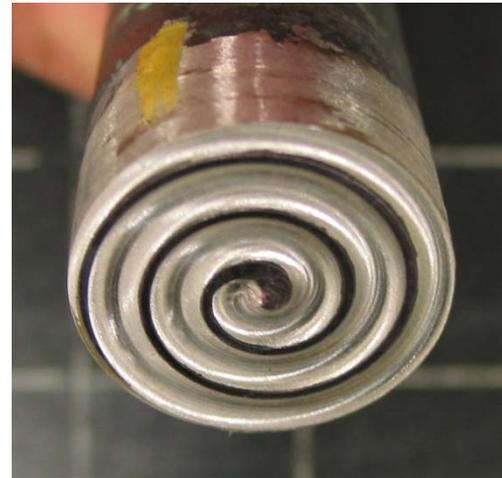
Very high levels of total strain are expected to produce extremely good mixing of constituents and potentially diffusion rates high enough for good oxide mobility and redistribution to form nanoclusters.
