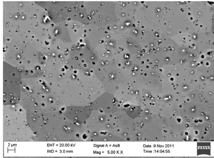
Significant coarsening of grains and oxides
