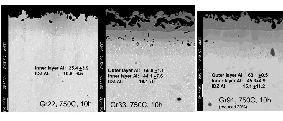
Apparent effect of Cr, but must consider as alloy system. Can heat treatment conditions produce a mechanically stable aluminide surface on Gr22?
