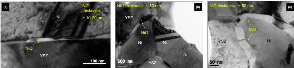
At a constant current of 0.3 A/cm<sup>2</sup>, (a) Cell operated in the 97% H<sub>2</sub> (with 3% H<sub>2</sub>O) for 196 h; and (b) and (c) Cell operated in the 24% H<sub>2</sub> (with 3% H<sub>2</sub>O and 73% N<sub>2</sub>) for 196 h. Both cells were cooled down nitrogen.
