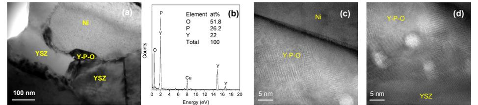
Y-P-O precipitate at Ni/YSZ/YSZ triple grain junctions for the cell operated in syngas/phosphine fuel for 110 h.
