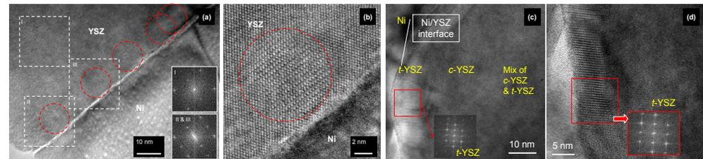
**Nanostructure and chemistry near Ni/YSZ interface for the cell operated in fuels containing phosphine for 120 h.**
