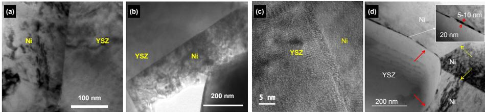
**TEM cross sectional view of:** (a), (b) and (c) Fully reduced button cells; and (d) Cell operated in hydrogen for 24 h (with 0.7 V of terminal voltage). Both cells were cooled down in nitrogen.
