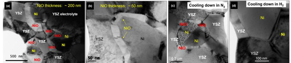
(a) Anode/Electrolyte interface of cell operated in H<sub>2</sub> containing 10 ppm PH<sub>3</sub> for 120 h. (b) Ni/YSZ interface of cell operated for 200 h. (c) Ni/YSZ interface of cell operated for 120 h cooled down in N<sub>2</sub>. (d) Cell operated for 120 h cooled down in N<sub>2</sub> with 1% H<sub>2</sub>.
