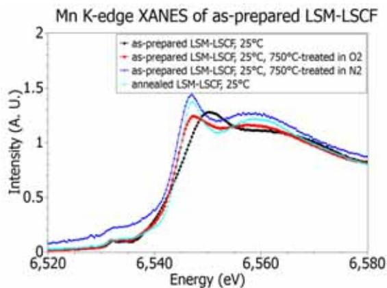
Regardless of atmosphere, the Mn edge shifts to lower energy with annealing at 750°C, indicating reduction in the oxidation state.
