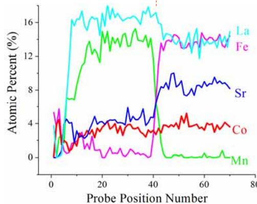
Samples are annealed at 850°C for 900 h
