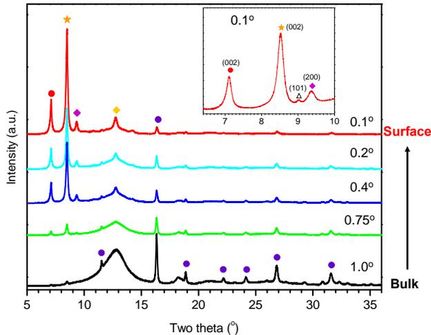
A gradient in oxidation state of cation along the thickness direction.
