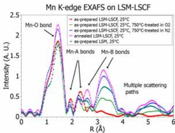
The peak growth and new features indicate ordering of the Mn local structure during annealing.
