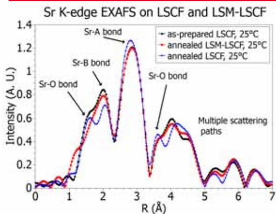
Peak splitting and peak shifting (at 2.8 Å) represent slight structural deformation, implying Sr segregation.
