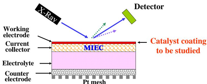
The information depth of XRA (to be bulk- or surface-sensitive) can also be tuned to varying degrees by using a combination of transmission spectroscopy and glancing angle geometries.
