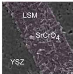
Raman mapping of SrCrO<sub>4</sub> on patterned LSM cathode exposed to Cr-containing vapor at 625°C for 24 hrs.
