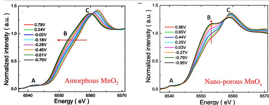
(a) *In-situ* XANES spectra showed an entire edge shift towards lower energy in a continuous manner, suggesting that the charge storage is mostly associated with the Mn<sup>3+</sup>/Mn<sup>4+</sup> redox reactions as conventionally believed. (b) The behavior of the nano-porous MnO<sub>x</sub> is different.
