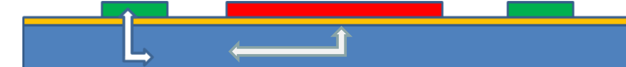
Fig. 6: Cross-section representation of Cell A, with the anode (blue), cathode (red) and ring electrode (green). The arrows show the presumed current flow for the cat/ring connection.
