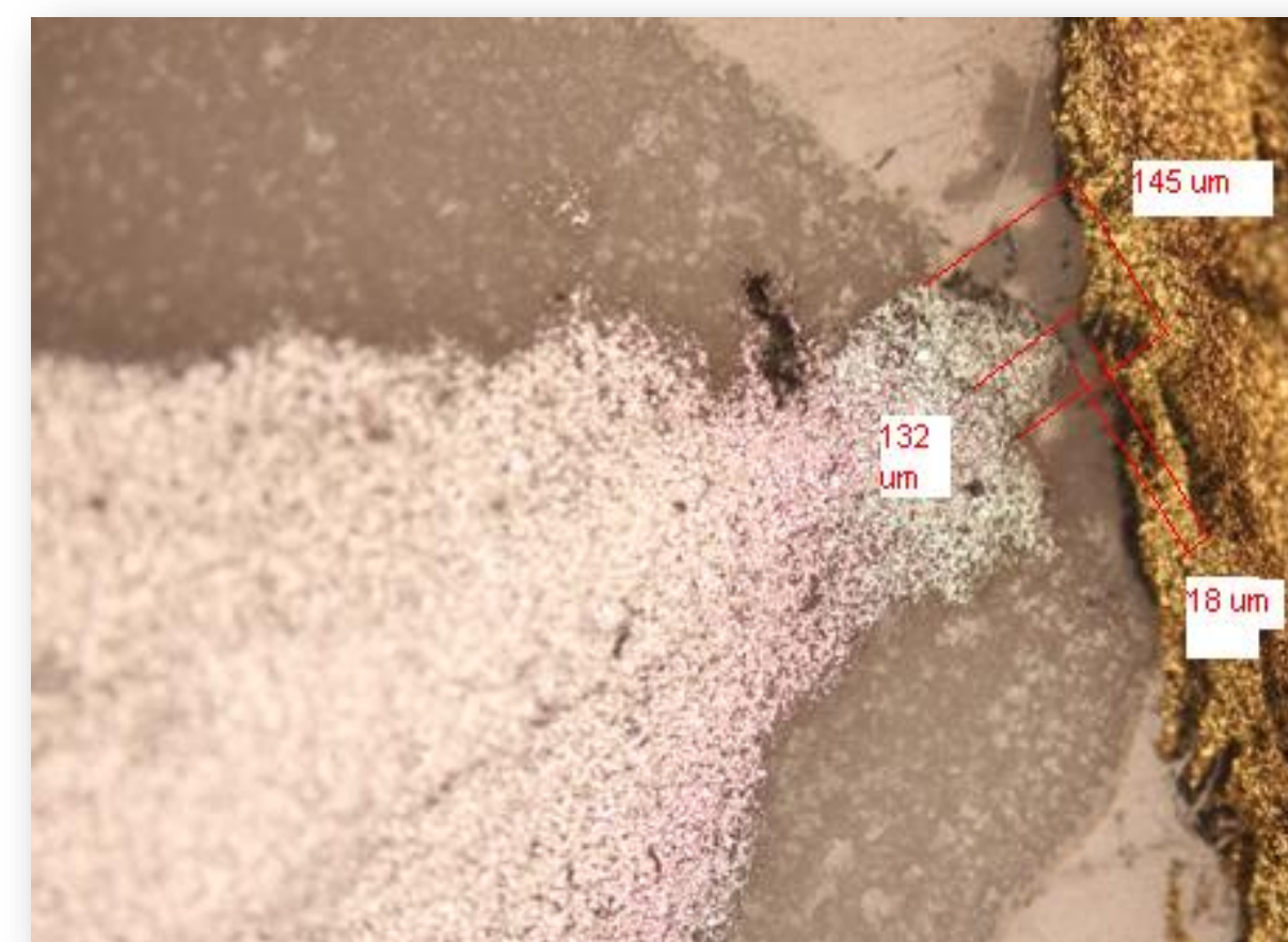
Fig. 3: Cell C, showing the gold paste-coated cathode (right side), the glass paste insulating pad (dark grey) and the silver paste reference electrode (bright silver).
