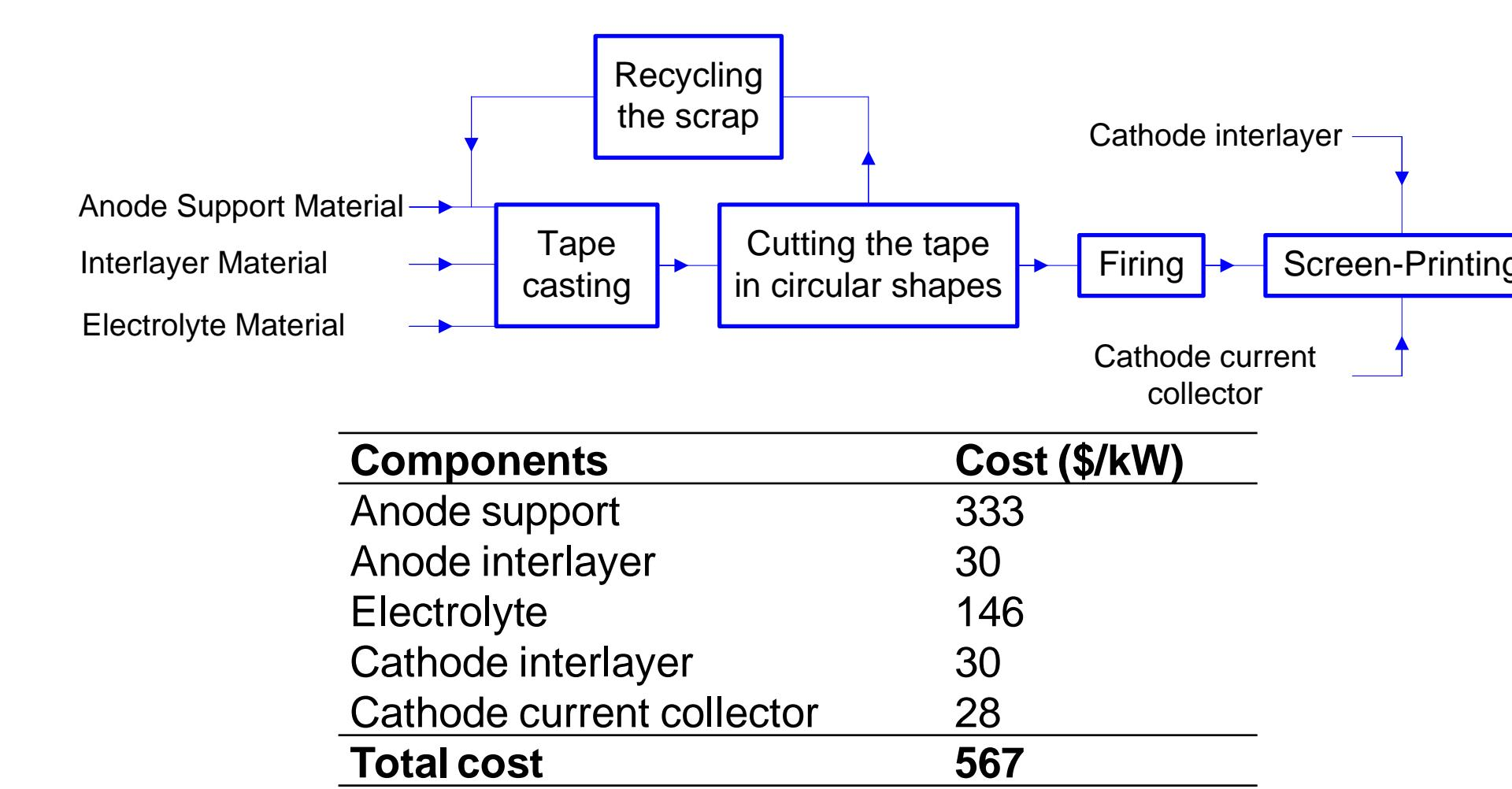
■ Fuel cell cost for generation of 1 kW electricity is about \$ 570.
