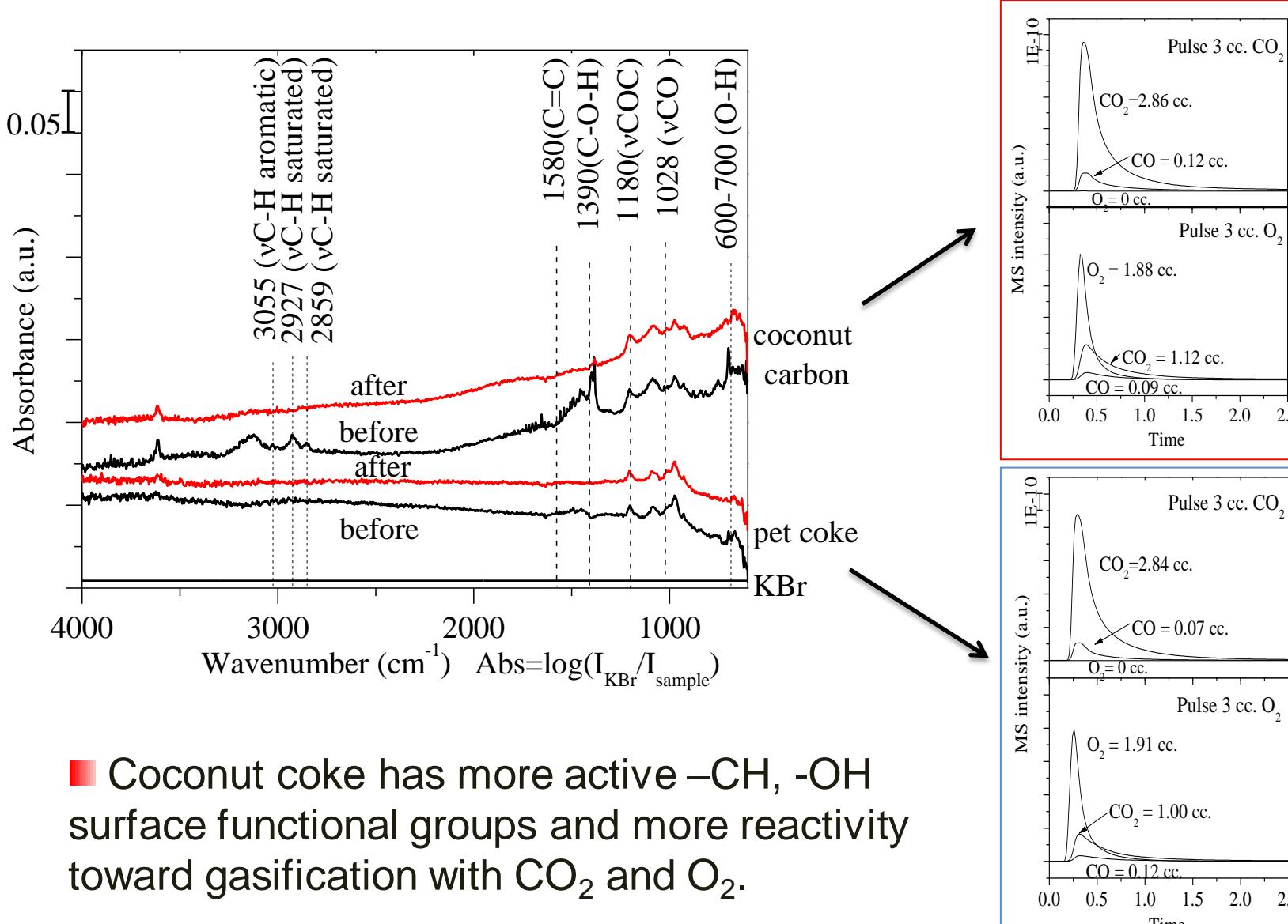
■ Coconut coke has more active -CH, -OH surface functional groups and more reactivity toward gasification with CO<sub>2</sub> and O<sub>2</sub>.
