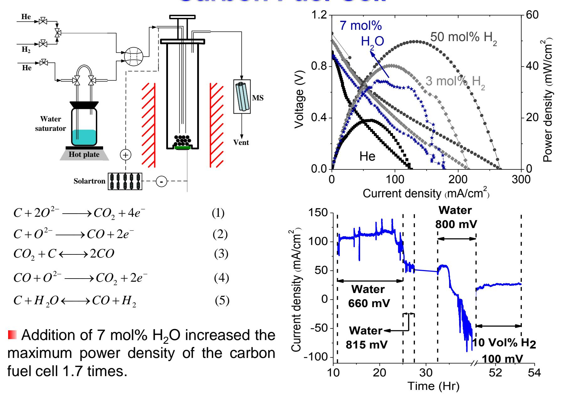
■ Addition of 7 mol% H<sub>2</sub>O increased the maximum power density of the carbon fuel cell 1.7 times.
