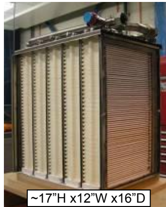
Block assembly (~20kW): 5 strips of 12 fuel-parallel bundles
