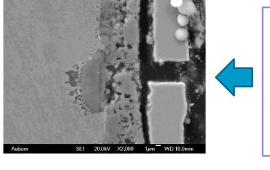
Coated H52 after 800 C-1600hr isothermal oxidation: Spallation of oxide scale was found. Cross section microstructure showed thicker oxide scale in some areas.
