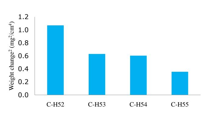
Weight change square after 800 C-800hr cycle oxidation (25hr interval)
