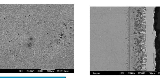
Coated H55 after 800 °C-1600hr isothermal oxidation: No spallation was found on the surface of the coating.
