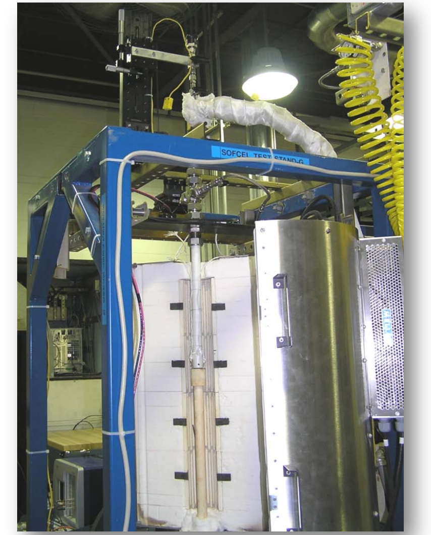
Test Sample Installed in Furnace
