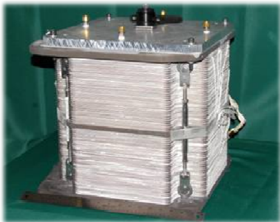
FuelCell Energy 64 cells 550 cm 2 active area
