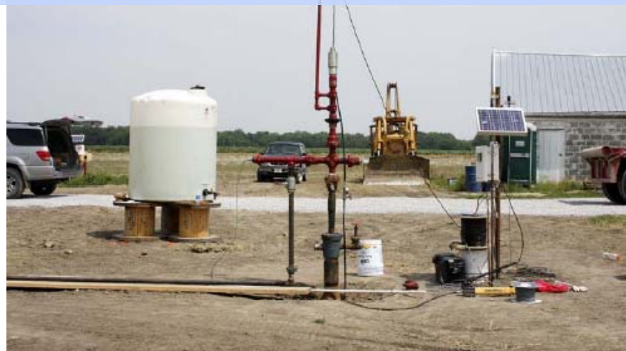
Injection Well with Monitoring Equipment at MGSC ECBM Test Site
