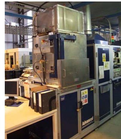
Rigs for QA testing of manufactured active substrates (2 of 4 scheduled install Aug '10)
