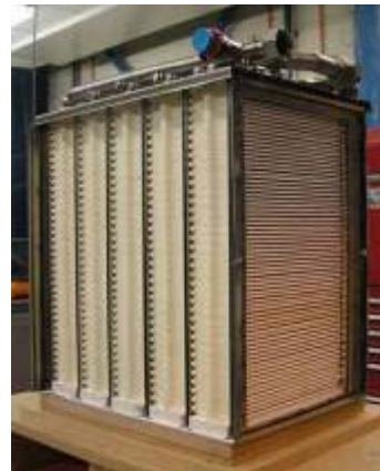
Block assembly, ~20kW (5 strips of 12 parallel bundles)
