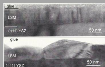
Top: As deposited films show ~30nm wide columnar grain growth. Bottom: Annealing at 1100°C for 4 hr introduces grain growth (~150 nm) and surface roughening.
