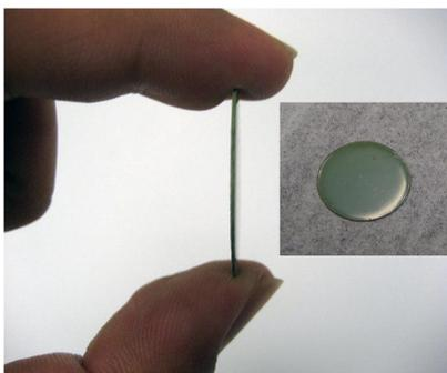
Co-sintered anode supported cell fabricated at WVU
