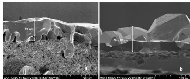
SEM micrographs of the top anode cross-section after exposure to dry  $\text{H}_2$  with 10 ppm  $\text{PH}_3$  at 800 °C. (a) The cell with 0.5  $\text{A cm}^{-2}$  load for about 120 h at 1000x magnification, (b) the cell without load for about 140 h at 500x magnification. The thickness of secondary phase layer is more for no (no  $\text{H}_2\text{O}$ ) load case.
