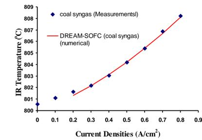
Model validation: Predicted SOFC surface temperature plotted along with measurements from in-situ experiments.
