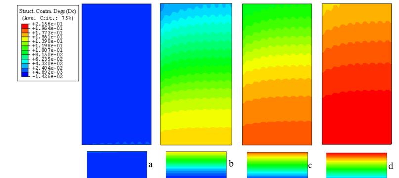
Predicted degradation of anode material in a planar cell due to contaminant along the fuel flow and across anode thickness under 5ppm  $\text{PH}_3$  exposure (a) 510h (b) 7410h (c) 12410h (d) 19410.
