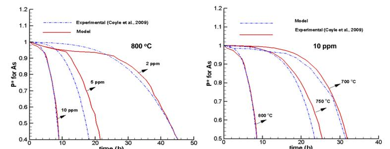
Predicted Performance degradation due to  $\text{AsH}_3$  exposure: Modified power density vs time at 0.05A/cm². Degradation model closely emulates the characteristic behavior of SOFC anodes at different temperatures and concentrations.
