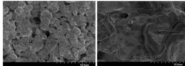
SEM images of the Ni/YSZ electrode surface (a) after 24 h of exposure to the clean syngas at 900 °C, (b) after 48 h of exposure to 10 ppm  $\text{PH}_3$  at 900 °C. Above images reveal that one possible reason for cell degradation due to  $\text{PH}_3$  is the effect P has on the anode microstructure.
