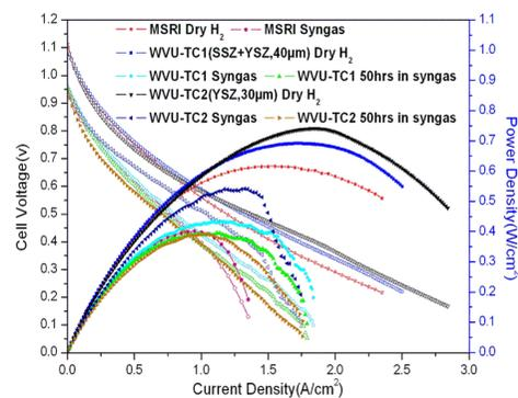
Button cells manufactured at WVU showed performance comparable to that of commercial cells
