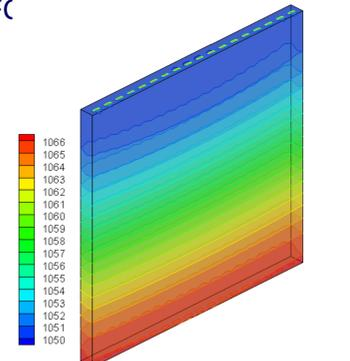
Predicted temperature distribution inside a counter-flow planar SOFC.
