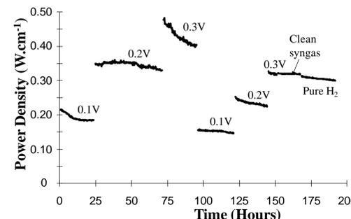
Power density vs time at constant cell voltage. Rate of power loss is not a definite function of the cell over voltage when cell is operated under syngas + 10 ppm  $\text{PH}_3$
