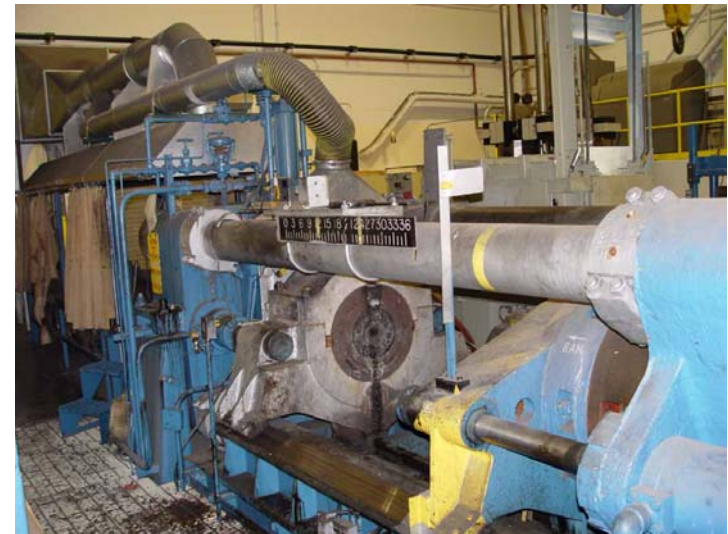
Watson-Stillman Co. (Roselle, NJ) unit with total capacity of 1,250 tons ( 2.5 \times 10^6 lbf)
