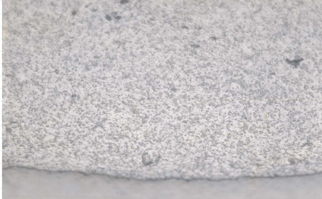
Bi-Metal Weldment 355 Stainless to 5083 Aluminum
