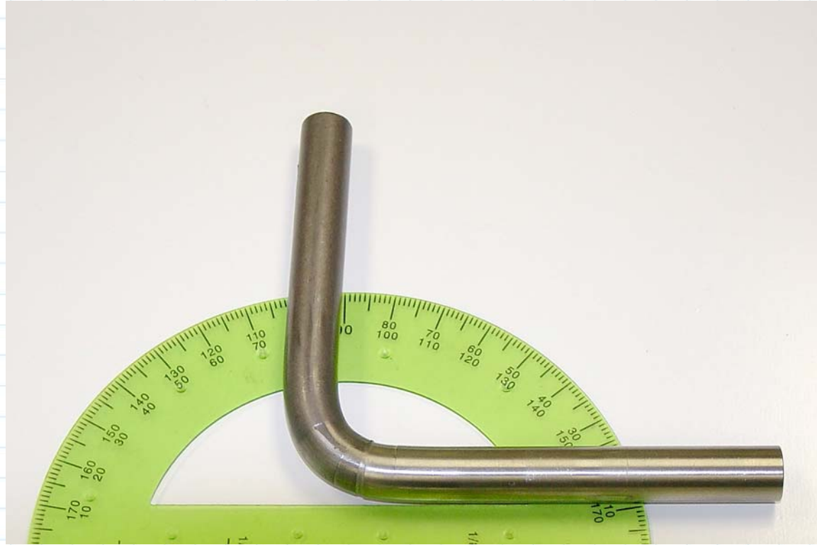
Tantalum to Niobium to Zirconium Bend Test
