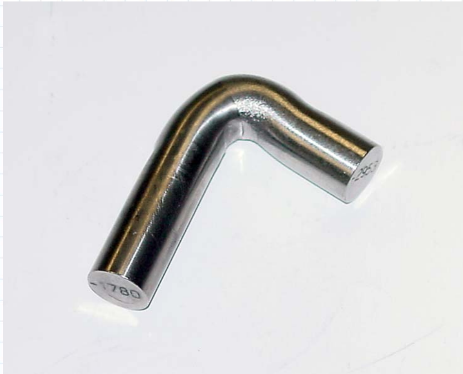
Titanium to Stainless Bend Test
