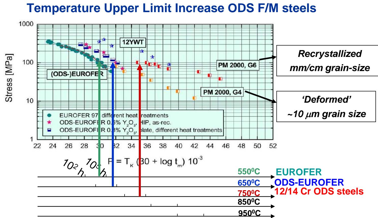
**Estimated Upper Limit on the Basis of a Creep strength of 100 MPa for ~50,000 Hours**
