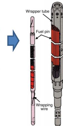
ODS fuel pin structure: BOR-60 irradiation test, proto-type FBR MONJU, Japan
