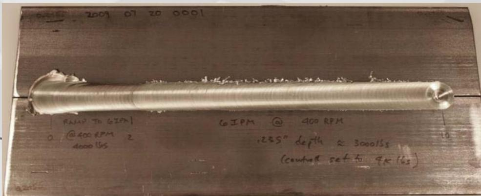
Full penetration, 300 mm long butt weld in 6.2 mm ( $\frac{1}{4}$ " ) thick plate
