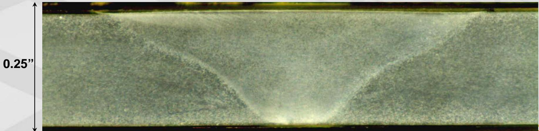
Fully consolidated, defect-free welds were made under a range of process parameters
