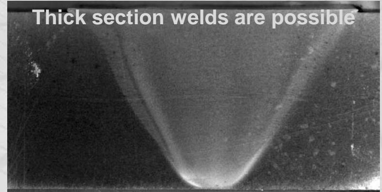
0.5" thick, single pass Friction Stir Weld in HSLA 65
