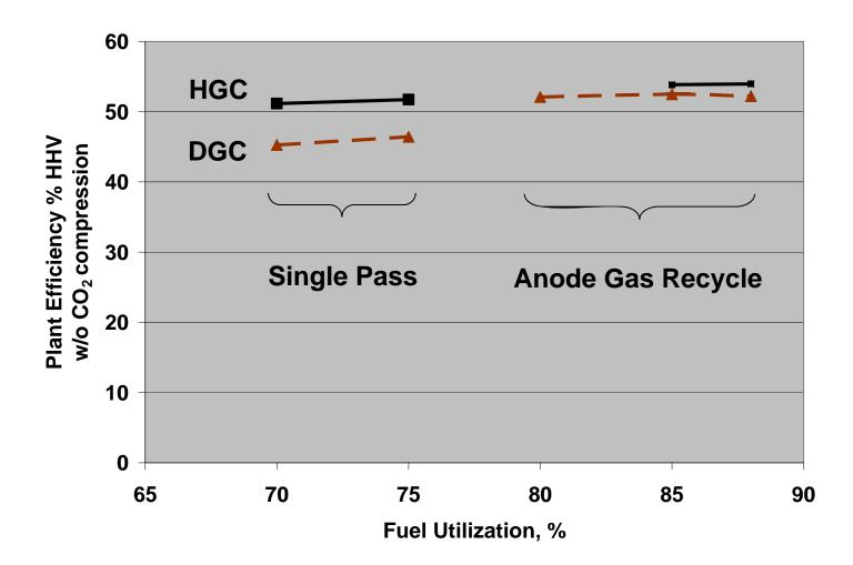
System: Catalytic gasifier; atm pressure SOFC; temperature: 650/800°C; DGC (dry gas cleaning) and HGC (humid gas cleaning); 50 mV voltage loss; CO<sub>2</sub> compression is 3.5 % points
