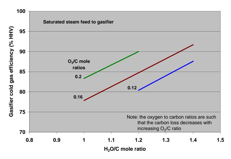
Cold gas efficiency for conventional entrained flow gasifiers: 75-80%
