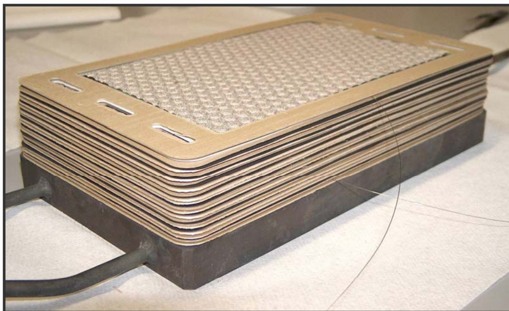
500-watt stack module (10 cells)
