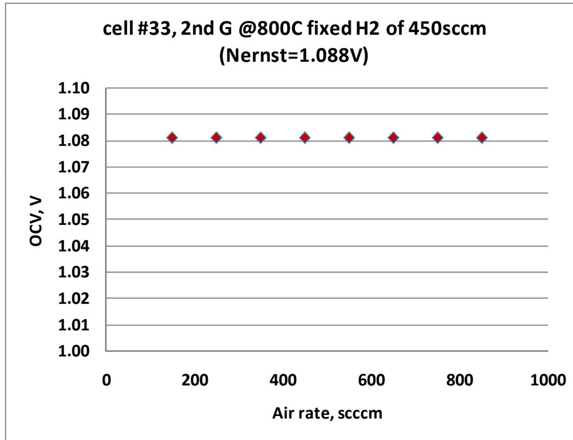
No cross-bubbling is consistent with insensitivity of OCV with varying air flow rate, indicating hermetic PEN/WF glass seal.
