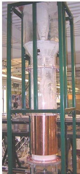
Flow structure in 4" and 12" fluidized beds with 60 \mu m FCC particles
