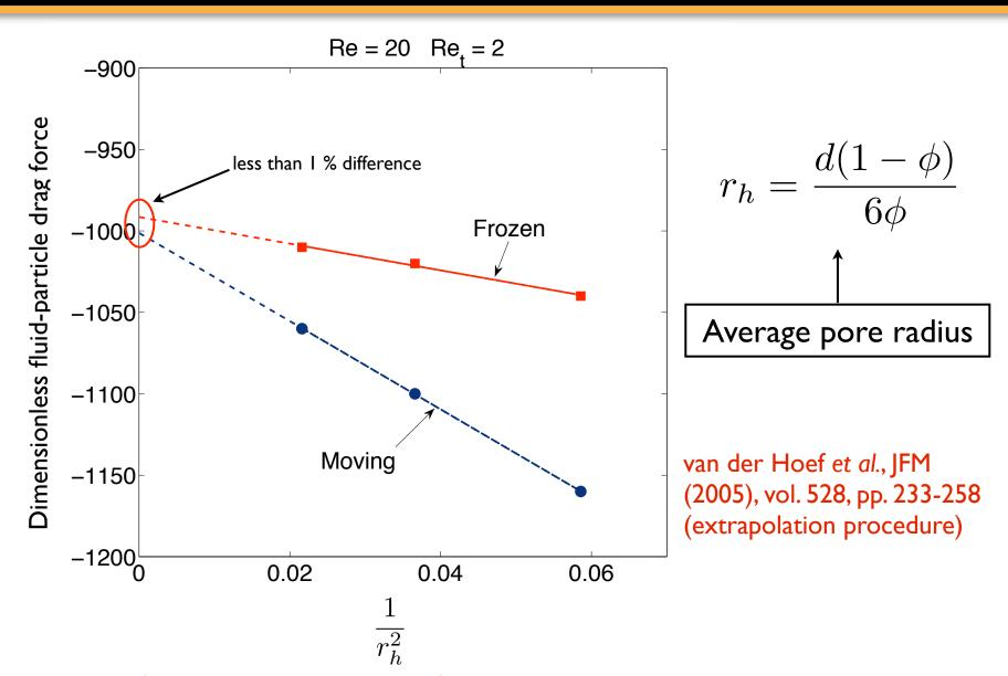
Must extrapolate frozen simulations to infinite resolution to get an accurate measure of the drag force in a moving suspension.
