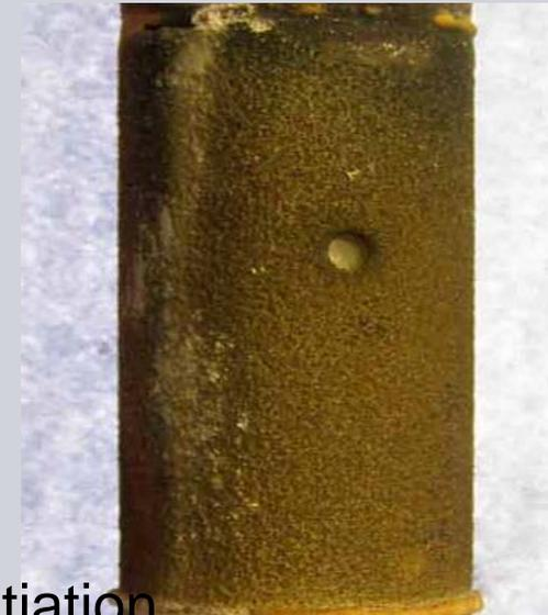
**Less severe damage of coated specimens compared to bare alloys**
