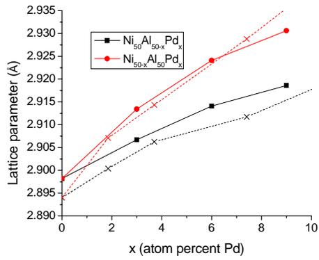
Figure 3. Lattice parameter variation with increased Pd content. The experimental values are indicated using solid lines and the theoretical values are indicated using dotted lines.
