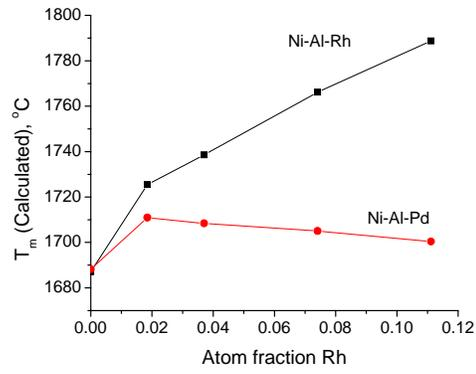
Figure 4: Variation of melting temperature with alloying additions
