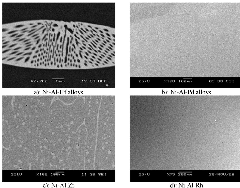
Figure 1. Microstructure of arc-melted, annealed ternary alloys: Ni-Al-M where M is a) Hf, b) Pd, c) Zr, and d) Rh
