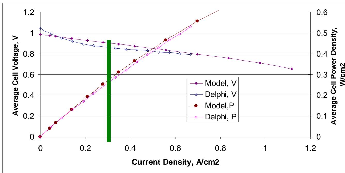
**Targeted Steady State operating point: 0.8 V/cell at 0.3 A/cm<sup>2</sup>**
