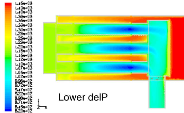
Contours of Static Temperature (K) Apr 18, 2008
