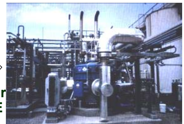
20kW DFC Operating on Destec Coal Syngas (4,000 hours) DOE-EPRI (1990 - 1992)
