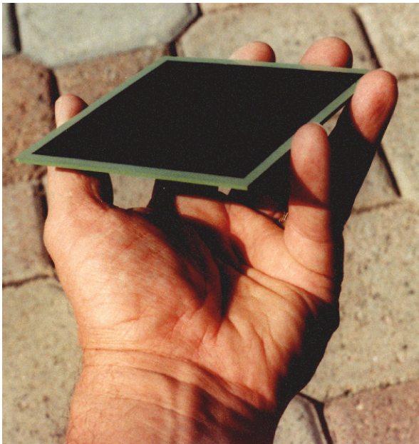
Anode Supported, Planar Cell Design
