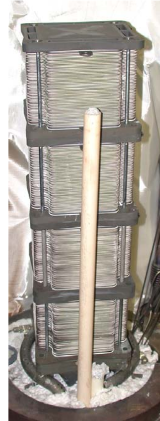
Stack Building Blocks Assembled Into Stack Tower
