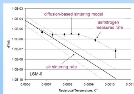
Sintering rates correlate with cation vacancy concentration changes in diluted air/oxygen alternated with nitrogen
