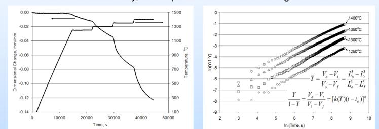
Enhanced sintering is attributed to the creation of a transient cation vacancy gradient as oxygen is gained and lost by LSM. For finite particles of radius  $a$ , that gradient is:
