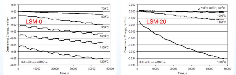
From isothermal dilatometry, kinetic parameters for air sintering are extracted
