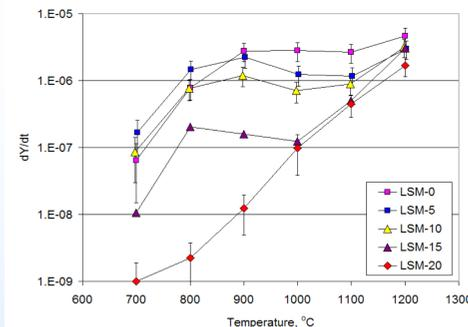
Dilatometry curves show high sintering rates for LSM-0 in alternating air/nitrogen for LSM, and negligible shrinkage for LSM-20, a widely used cathode material
