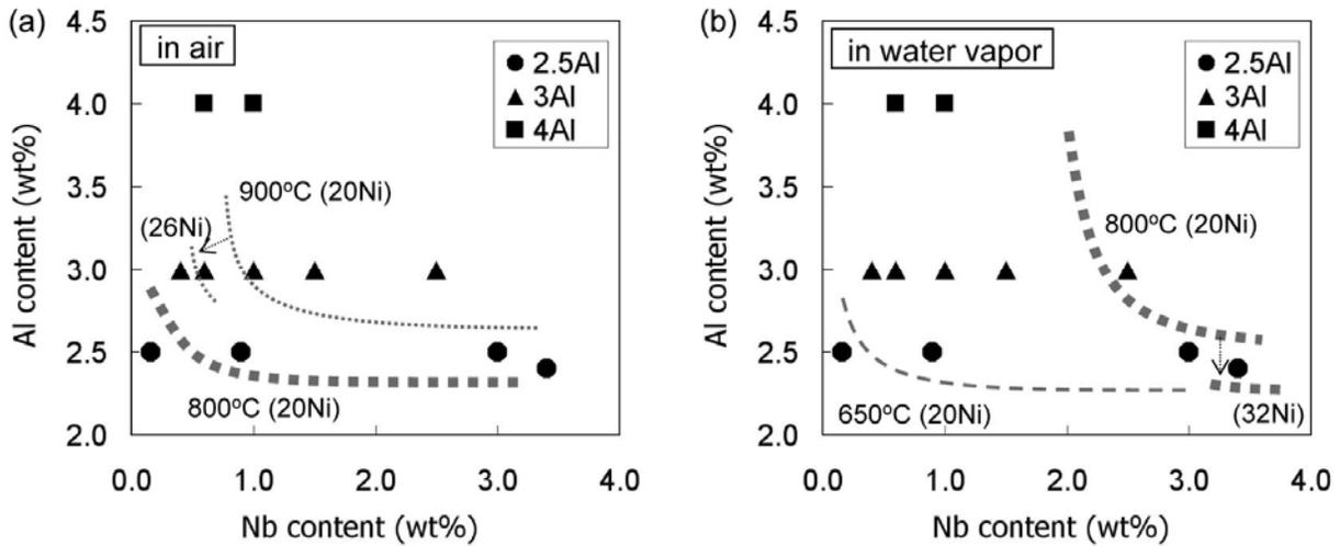
Fig. 2- Composition maps of alumina formation as a function of Al and Nb level in (a) air and (b) air with 10% water vapor.
