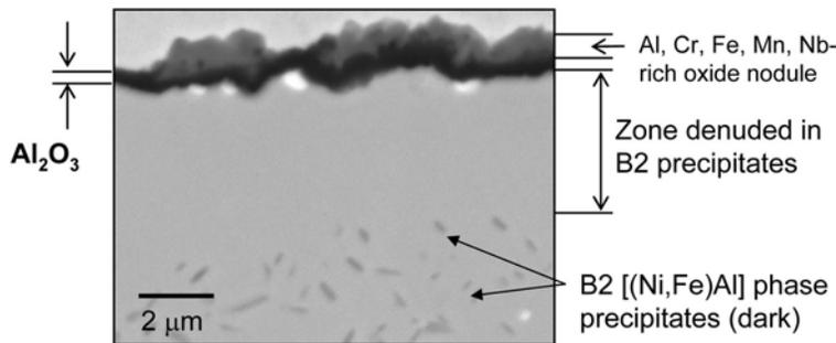
Fig. 3- Backscattered electron image of AFA 4-1 (4Al/0.6Nb/0.1Ti) after 100 h at 900 °C in air (after reference 7).
