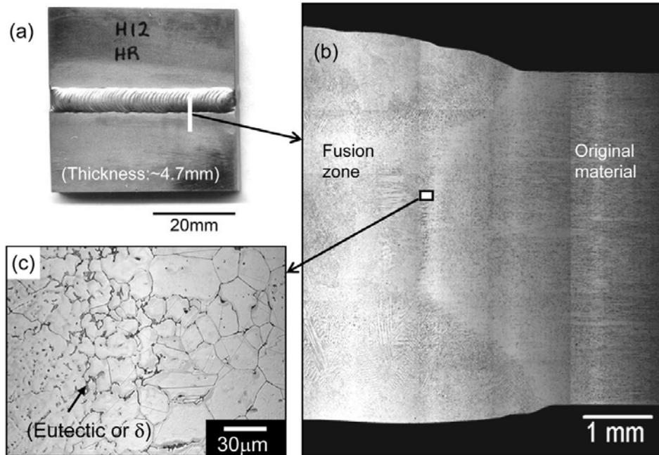
Fig. 7- Weldability screening of vacuum cast and hot-rolled AFA 4-1 (4Al/0.6Nb/0.1Ti) by gas tungsten arc welding using AFA 4-1 filler (after reference 2): (a) overall view, and (b and c) optical micrographs of cross-sections.
