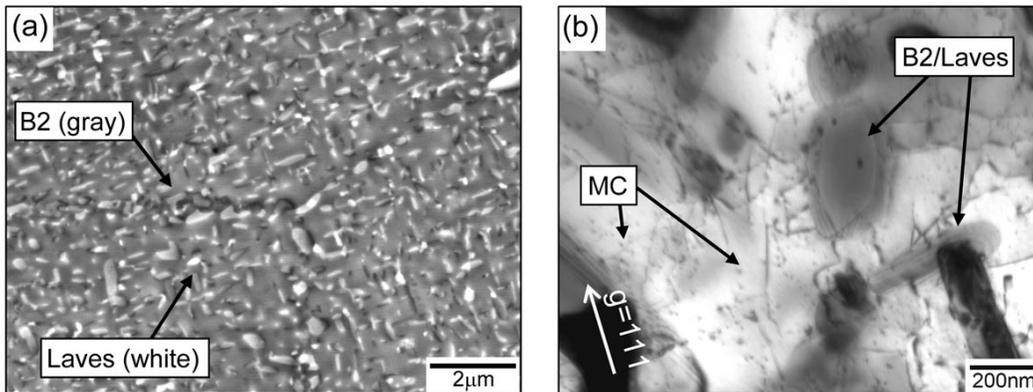
Fig. 6- Microstructure of creep-ruptured AFA 3-2 (3Al/0.6Nb/0.1Ti) tested at 750 °C and 170 MPa: (a) SEM back-scattered electron image and (b) TEM bright field image.
