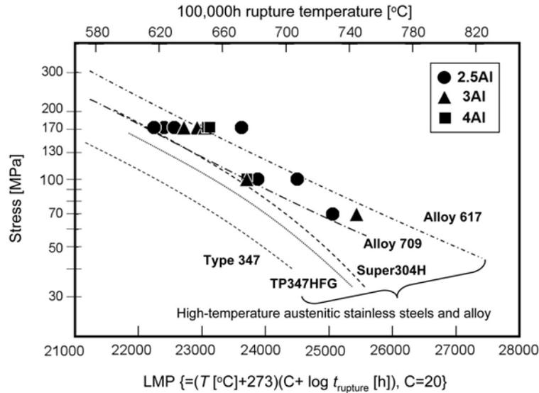
Fig. 4- Larson Miller parameter plots of the AFA alloys creep-rupture tested at 750 – 850 °C, together with those of heat-resistant austenitic steel alloys (after reference 1-4, 6, 8, 18-20).
