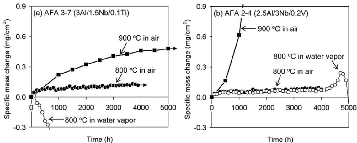
Fig. 1-Oxidation kinetics at 800/ 900 °C in air or in air with 10% water vapor: (a) AFA 3-7, and (b) AFA 2-4 (after reference 7).
