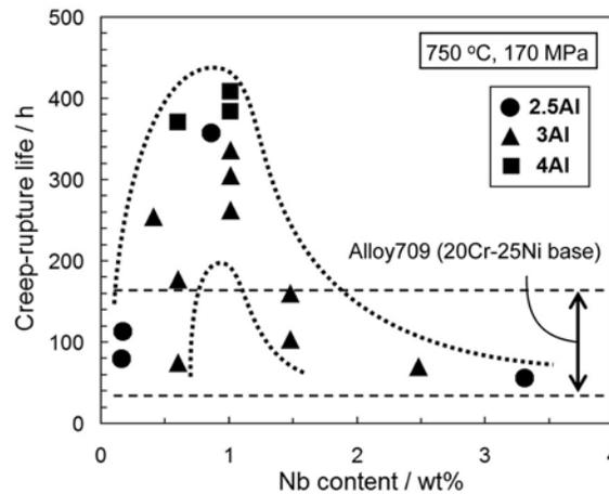
Fig. 5- Creep-rupture life data for the AFA alloys at 750 °C and 170 MPa in air plotted as a function of the Nb content (after reference 8). The dashed lines correspond to the creep-rupture of alloy 709 (no prior cold work) extrapolated to these test conditions [22].
