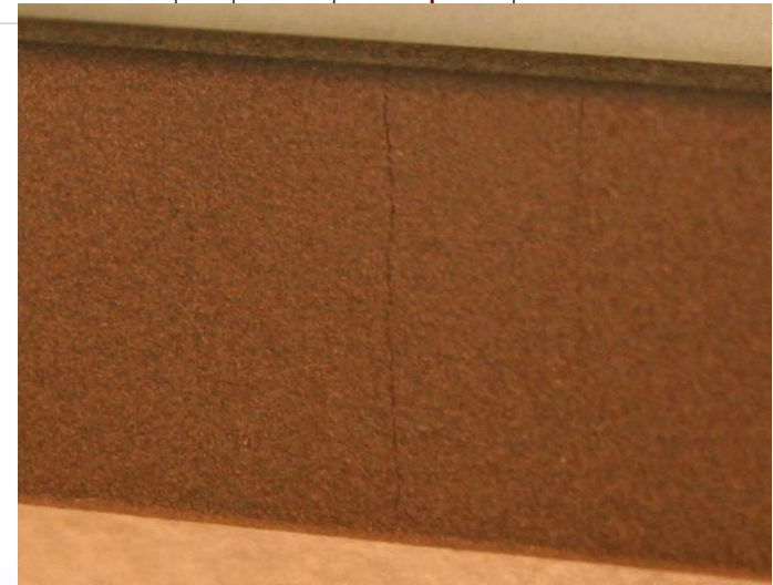
Eddy Current Detection of Cracking in a Coating
