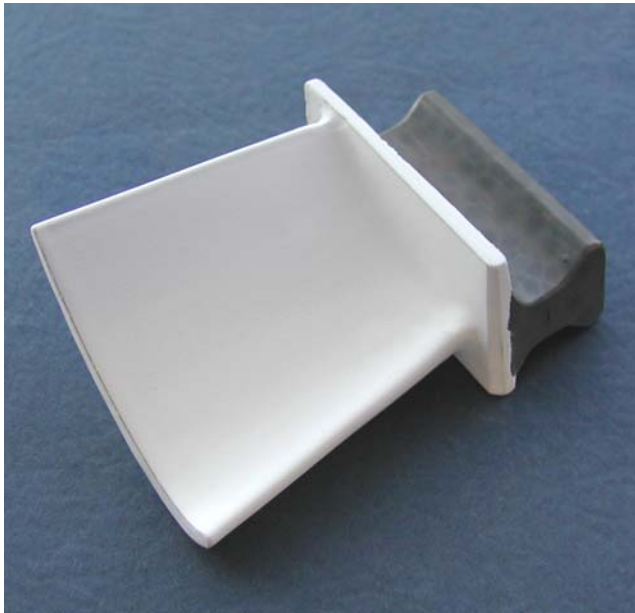
Rare earth silicate coating on a complex-shaped component (NT154 Si 3 N 4 Blade)
