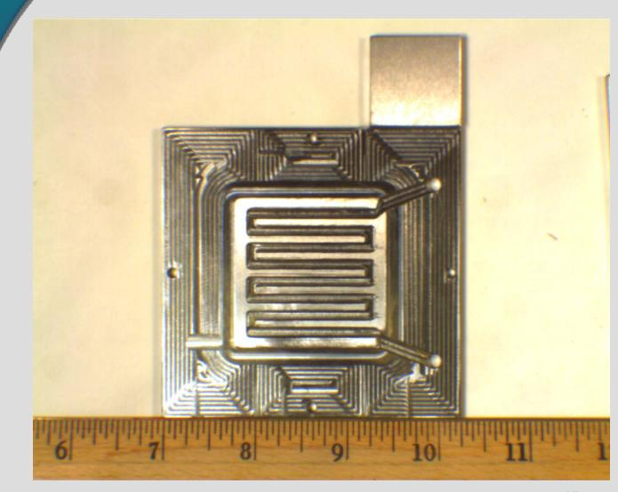
4.5 mm thick441 steel(coated withMn-Cospinel)
