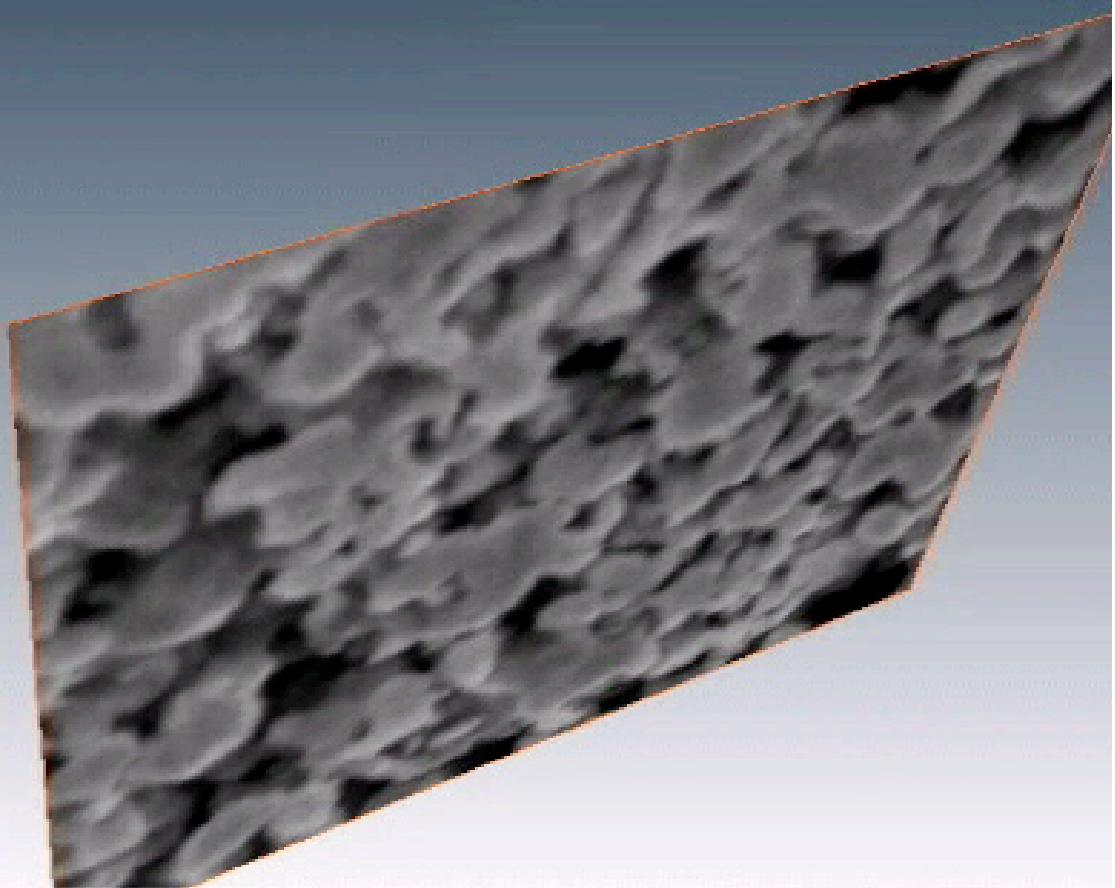
Dual beam FIB/SEM serially sections, and images porous SOFC cathode at 20nm intervals
