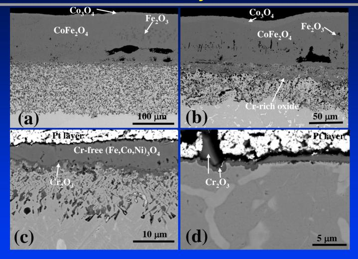
Cross-sections of the alloys with different X levels after oxidation for 3 weeks: (a) 0; (b) 0.75; (c) 1.5; (d) 3.5
