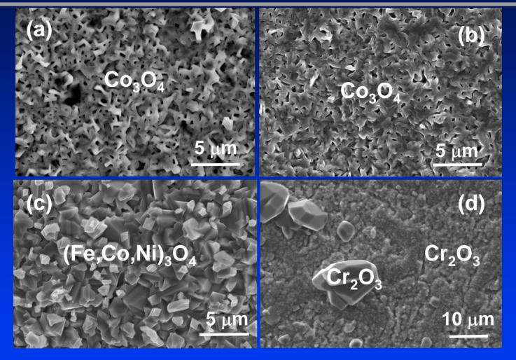
Surface morphologies of the alloys with different X contents after oxidation for 3 weeks (a) 0; (b) 0.75; (c) 1.5; (d) 3.5
