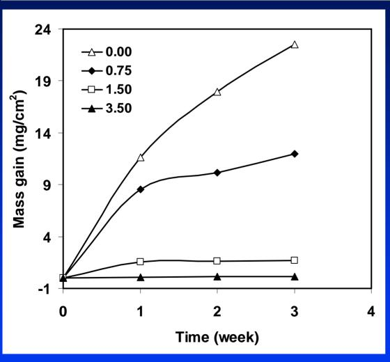
Oxidation kinetics of low-Cr Fe-Ni alloys with different X levels at 800°C in air
