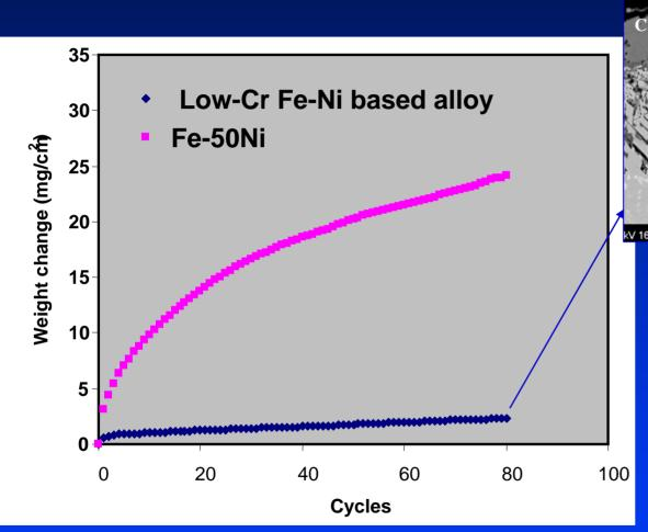
Oxidation kinetics of two Fe-Ni alloys after 80 cycles (25-h cycle, 800°C, air cooling)
