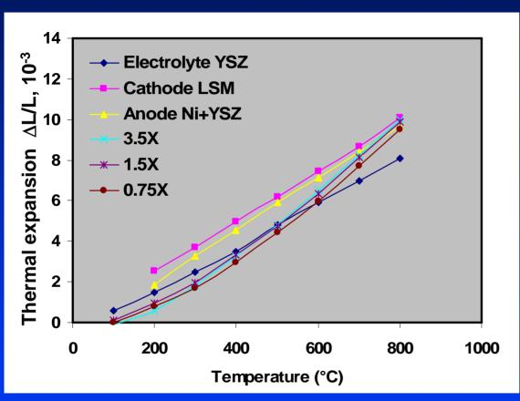
Thermal Expansion vs. Temperature for the Low-Cr Fe-Ni Alloys (wt.%), as Compared to Other Cell Components
