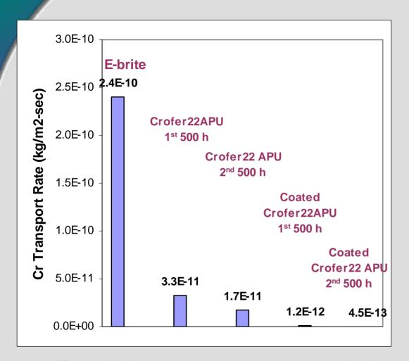
Cr release of coated Crofer22APU was <4% of Cr release of uncoated Crofer22APU
