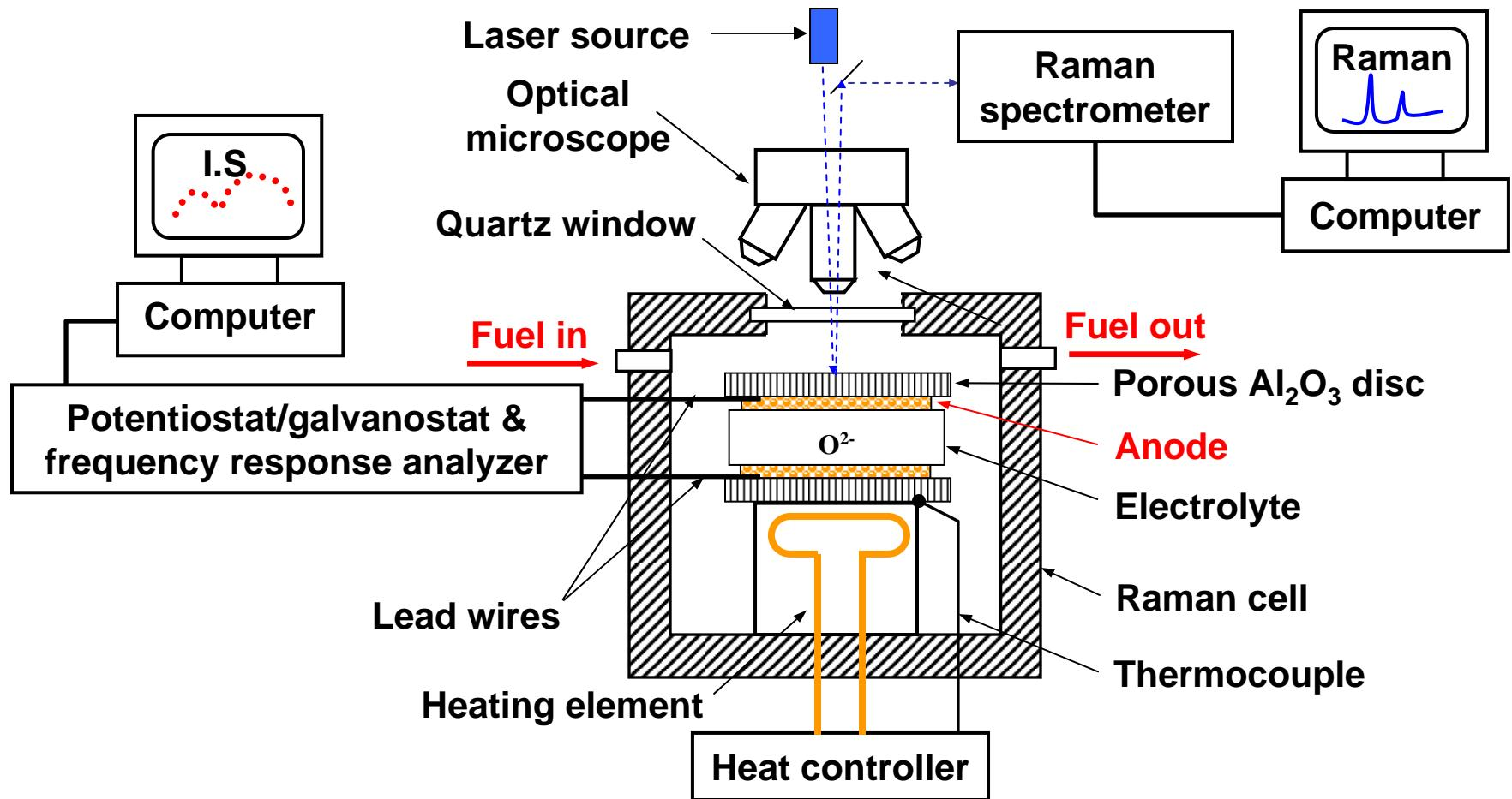
Schematic for the experimental setup of *in-situ* Raman spectroscopy coupled with electrochemical characterization instruments
