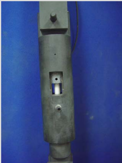
Creep testing of G18 glass to measure long-term deformation behavior
