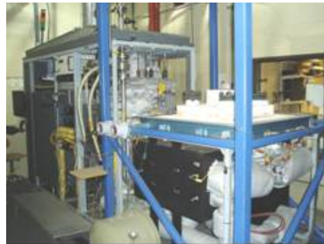
Test Facility For Regen HX and Anode Recycle Blower Evaluation
