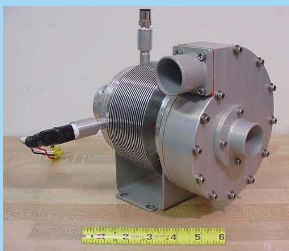
Automotive PEM Reformer Air Blower
