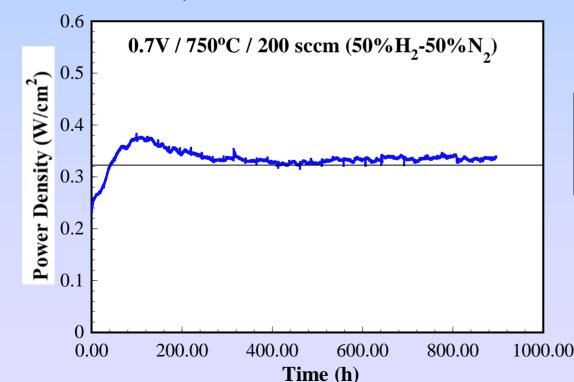
LSM-SDC mixed cathode with SDC interlayer. Au mesh/paste current collector.
