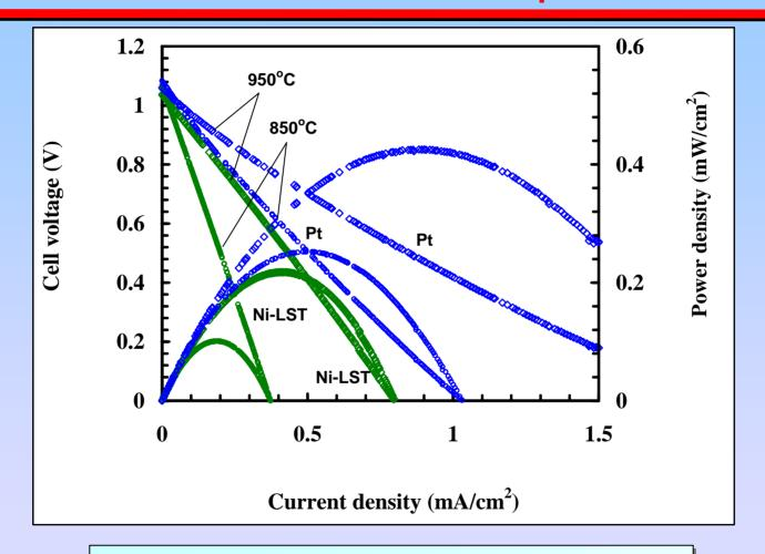
160 μm YSZ electrolyte-supported cell (La,Sr)TiO<sub>3</sub>- Ce(La)O<sub>2</sub> anode and LSF20 cathode with SDC interlayer; Fuel: H<sub>2</sub>/H<sub>2</sub>O=97/3; Oxidant=air
