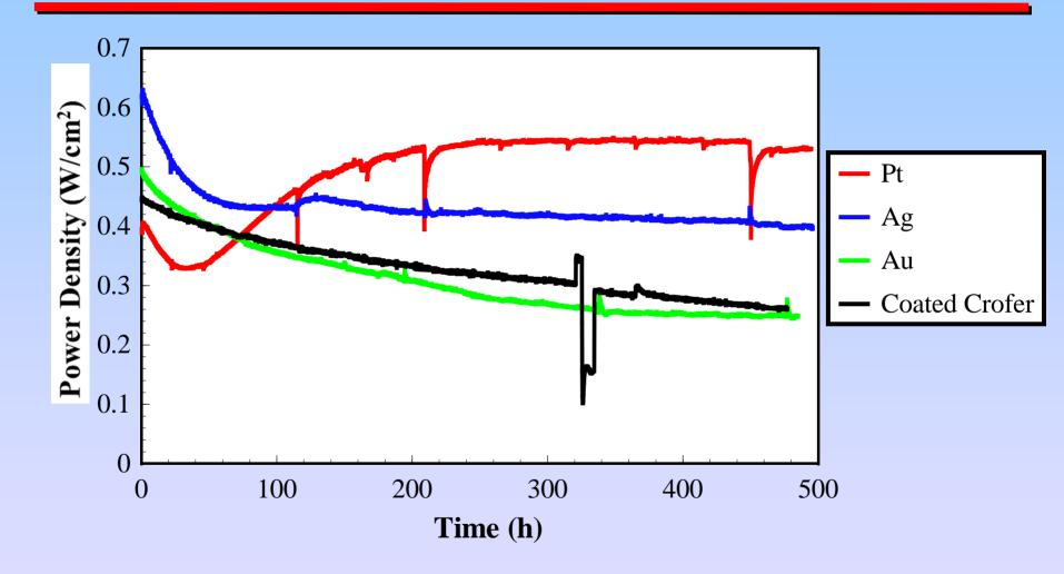
Anode supported cells tested on 50/50 H<sub>2</sub>/N<sub>2</sub>; 750°C; 0.7 V
