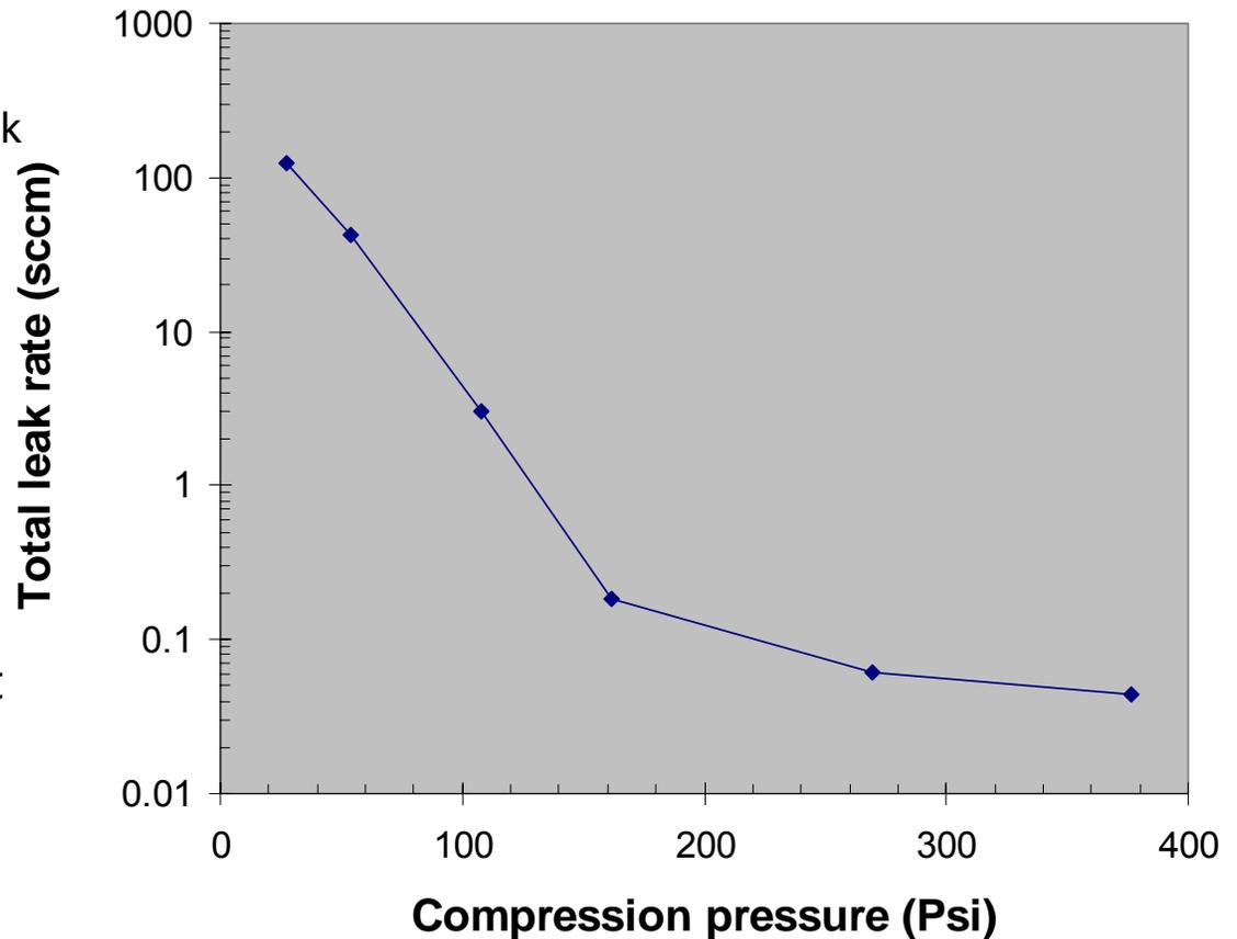
Gas leaks primarily through the interfacial path; leak rate through the bulk is about 4 order of magnitudes lower !!
