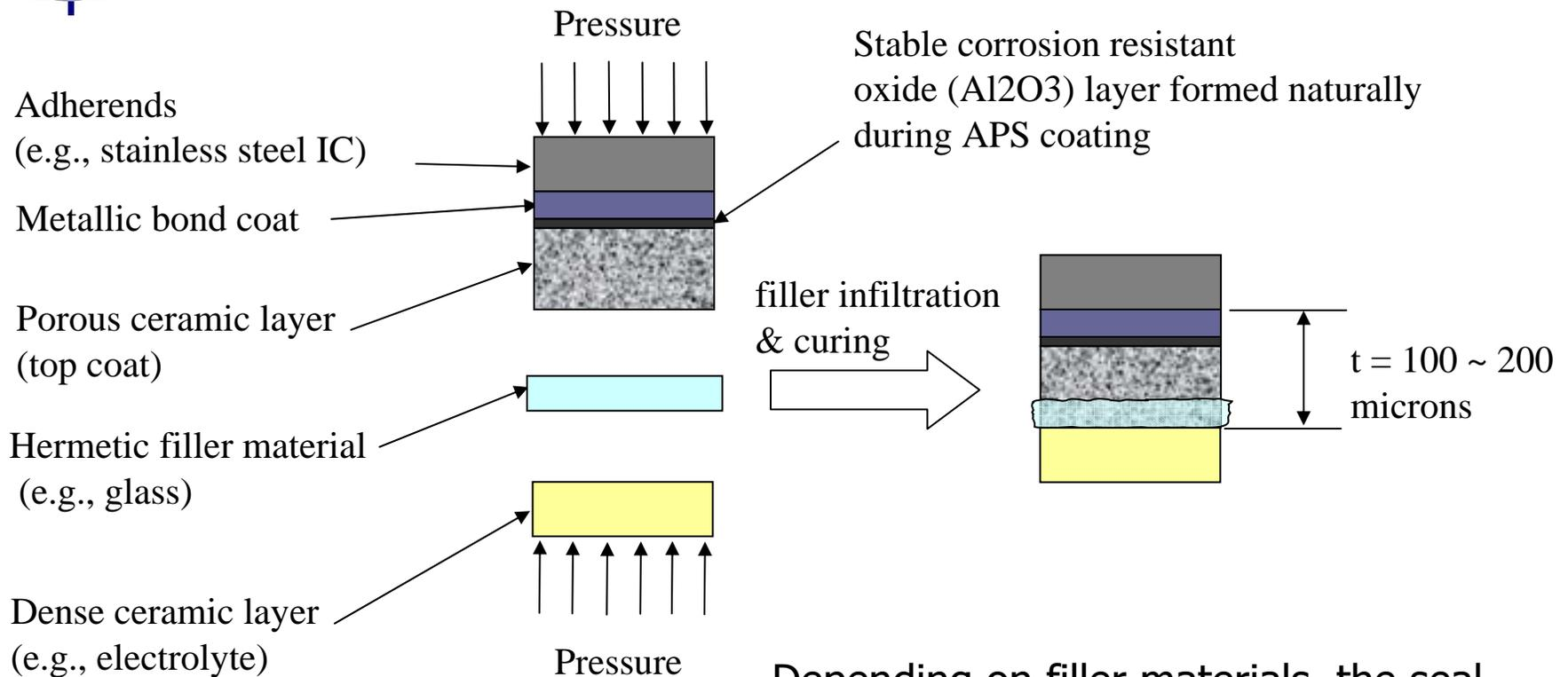
Depending on filler materials, the seal structure can be made either rigid (hard, solid) or compliant (soft, wet)
