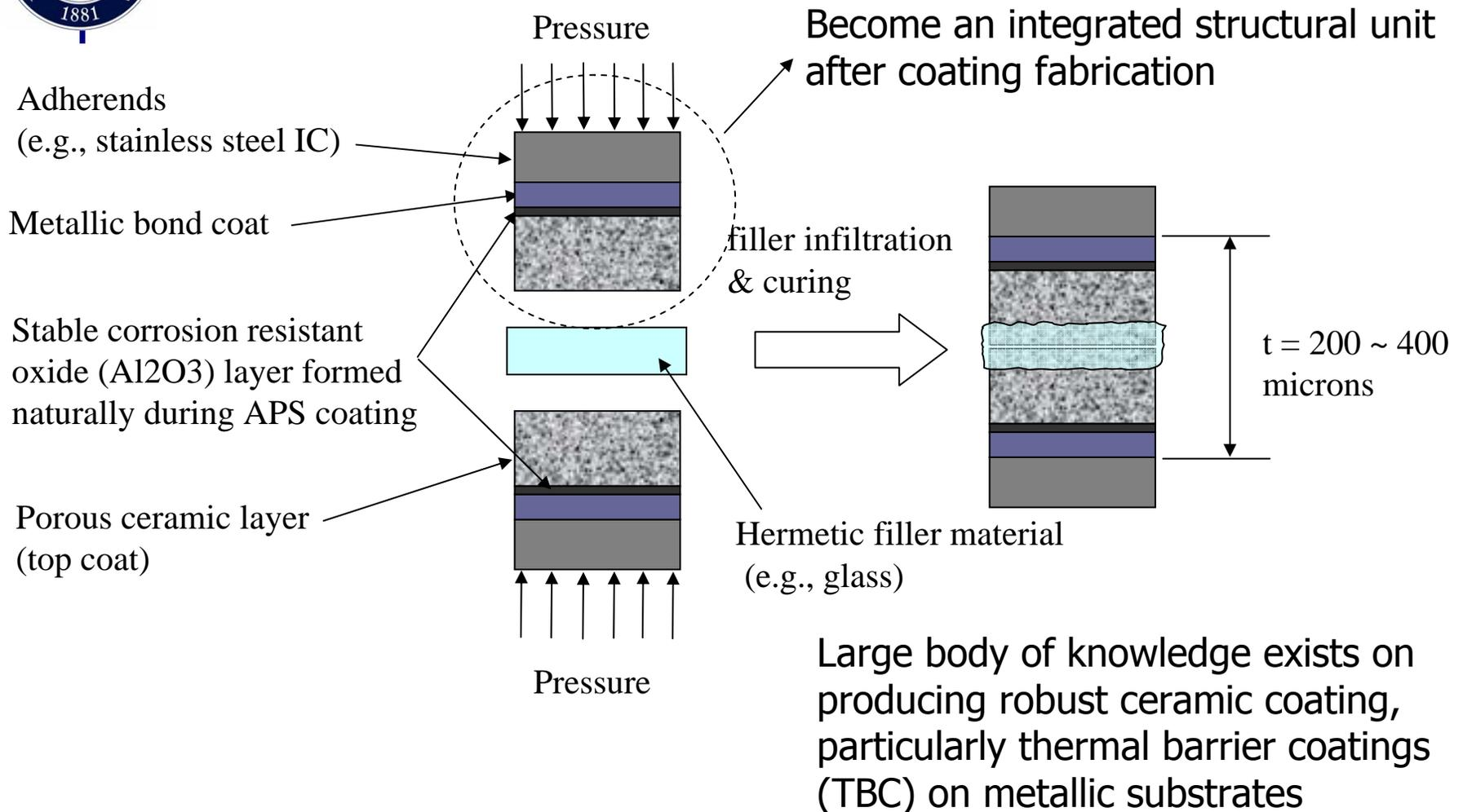
Large body of knowledge exists on producing robust ceramic coating, particularly thermal barrier coatings (TBC) on metallic substrates
