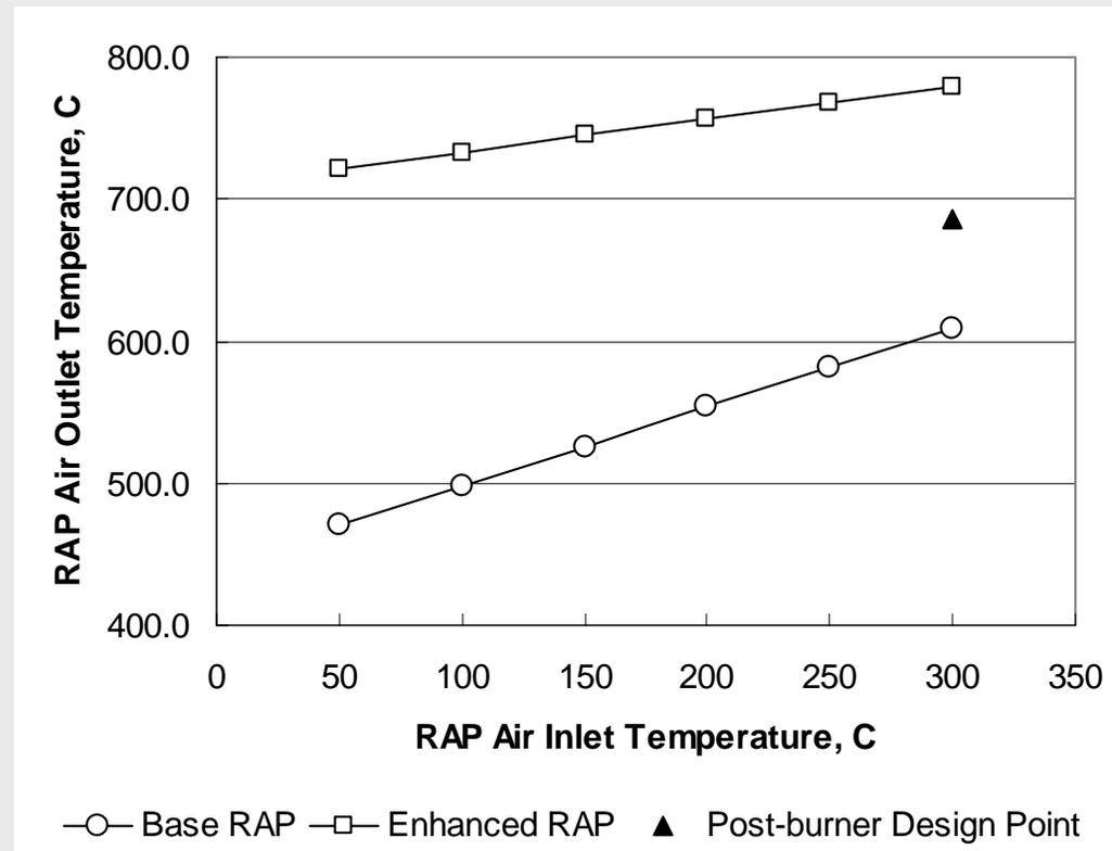
**Enhanced design: steel wool inserted between RAP walls**
