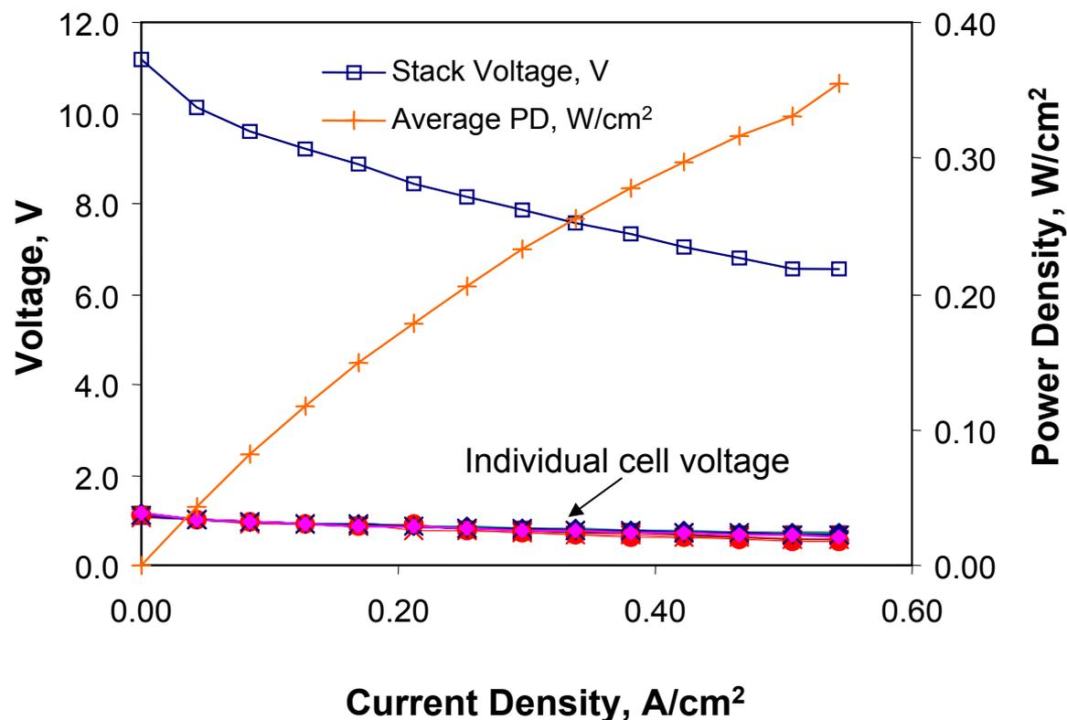
**355mW/cm<sup>2</sup> (6.6 @ 0.542A/cm<sup>2</sup>) with 64% H<sub>2</sub> at 800°C and 36.5% fuel utilization (total power output 500 W);**
