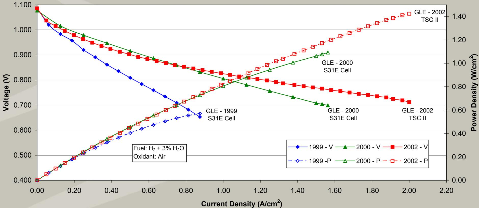
***Cell performance for a 10 x 10 cm<sup>2</sup> cell using stainless steel current collectors, cross-flow gas delivery***
