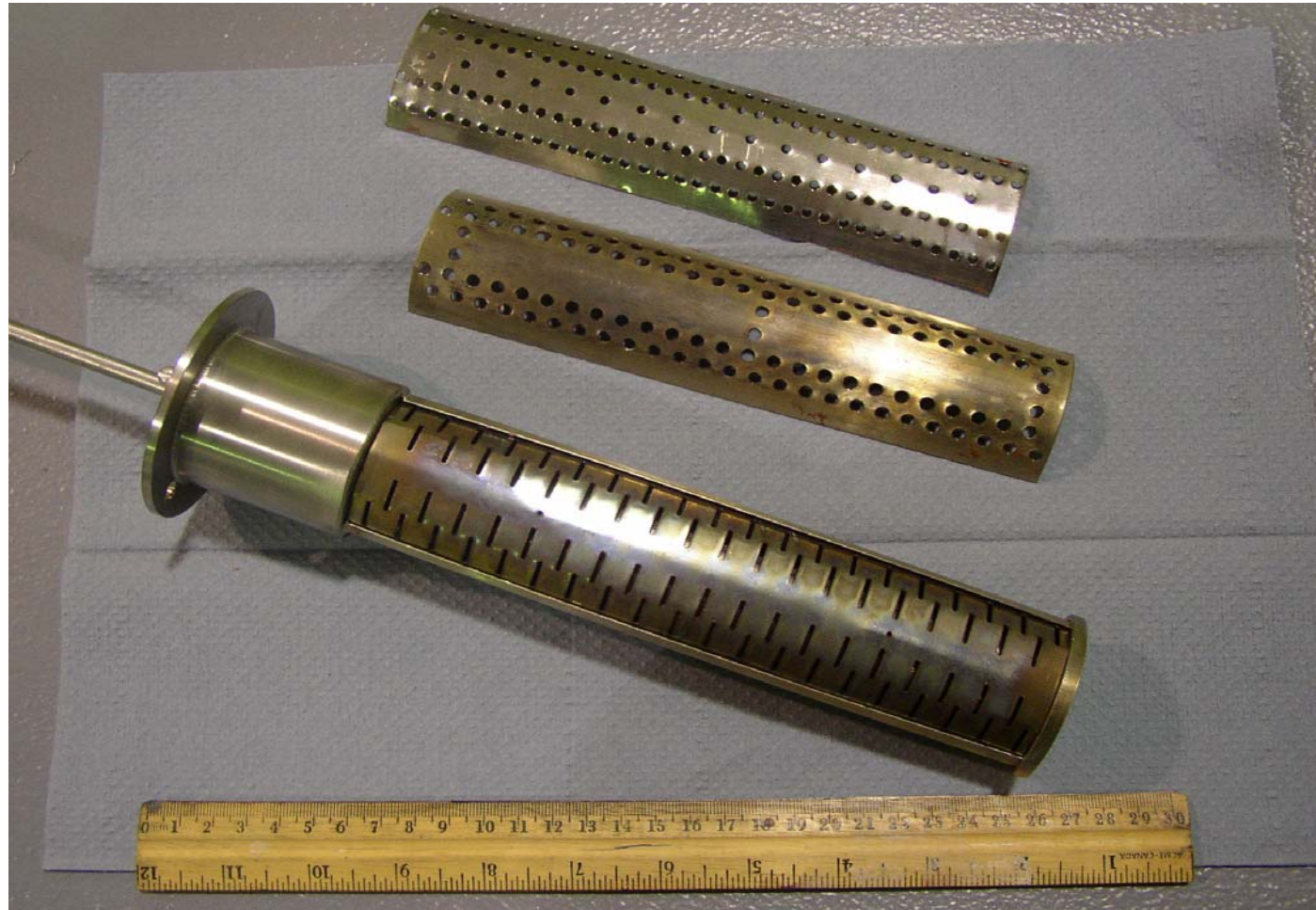
Prototype Combustor and Flame Holder Designs
