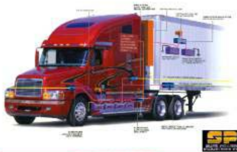
Heavy Duty Truck APU to eliminate long term idling: Diesel fuel
