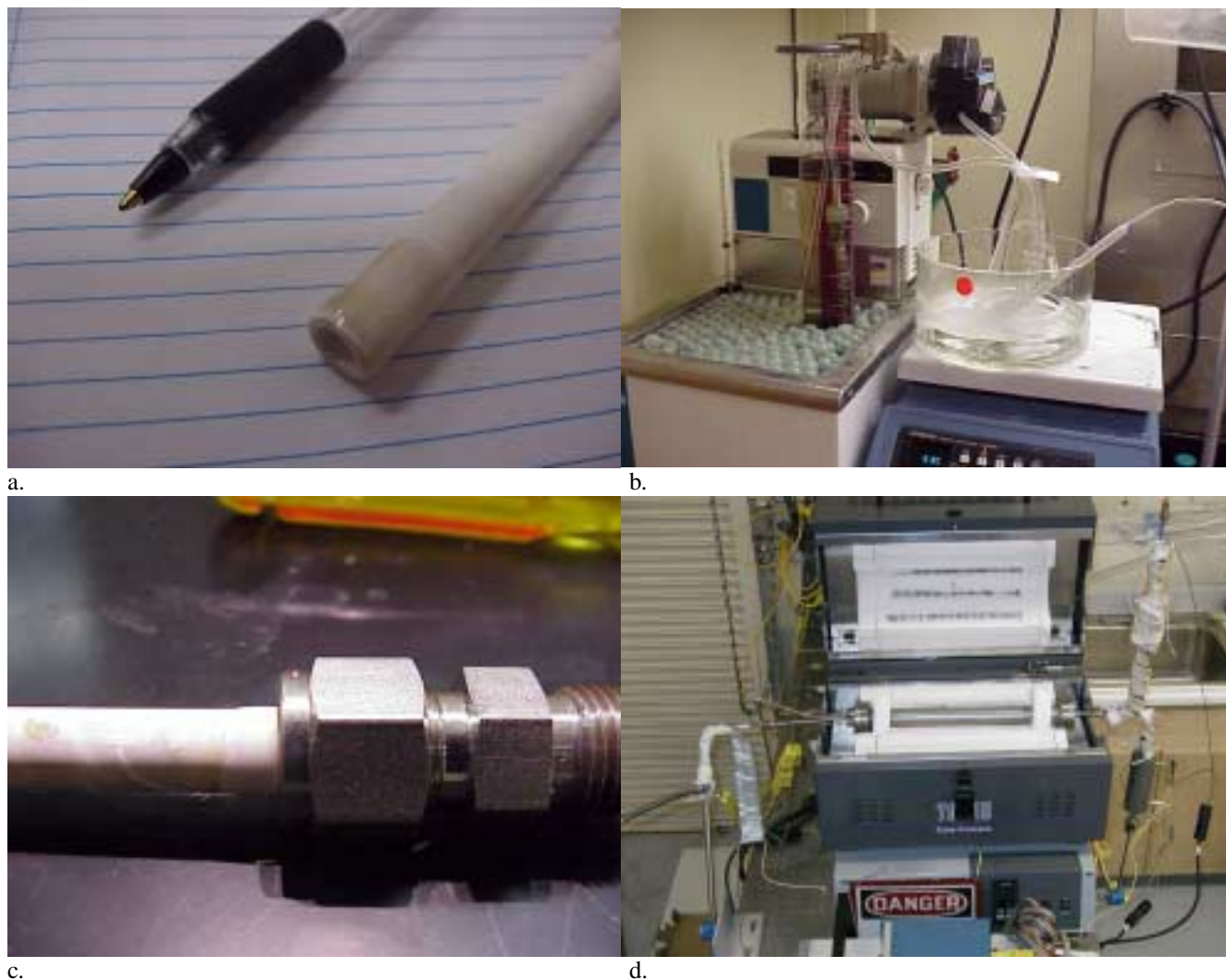
Figure 2. (a) glazed end of \alpha -alumina membrane (b) flow-through electroless plating system (c) SS compression fitting with graphite ferrule (d) test furnace with membrane module.
