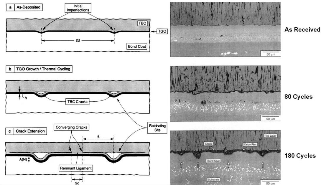
Fig 1. Schematic diagram and optical photomicrographs showing changes in topography between TGO and substrate for EB-PVD TBC(After Evans, et al 1997)
