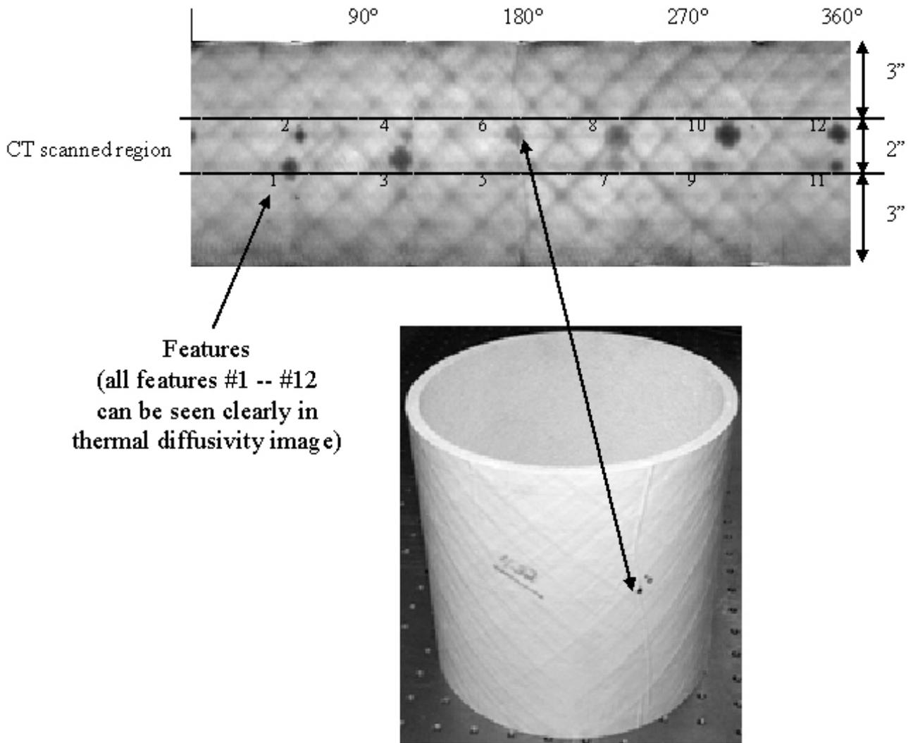
Figure 7. Example of detection of delaminations of sample shown in Fig 6. The thermal image data are obtained using one-sided acquisition parameters
