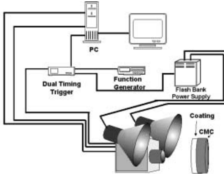
Fig 5. Schematic diagram of the one-sided thermal imaging NDE method for delamination detection for EBC.
