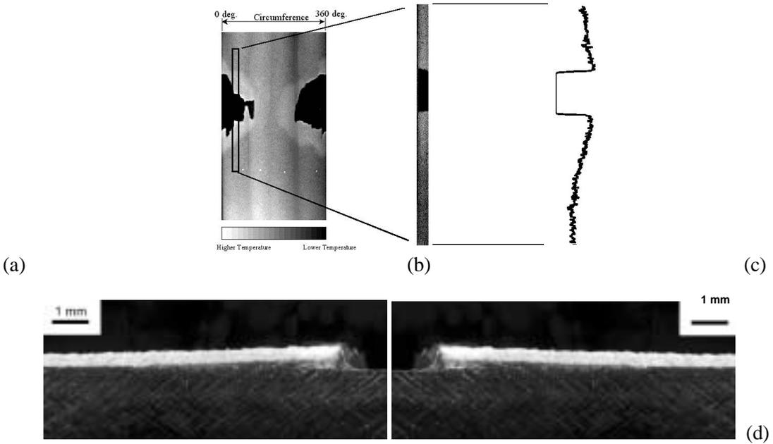
Fig 4. Example of polarized-laser back scatter for detection of de-bonds in APS TBC. a) One-sided thermal image showing delamination and laser scan position, b) laser scan data, c) line plot of laser scan data, d) optical photomicrographs of delaminated region.
