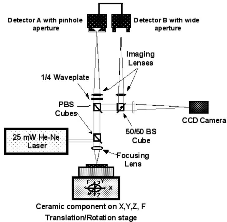
Fig 2. Schematic diagram of the polarized laser back-scatter NDE method for studying the topography of the TGO-substrate interface.
