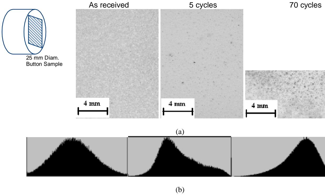
Fig 3. Polarized laser back-scatter data from thermally cycled EB-PVD samples.
