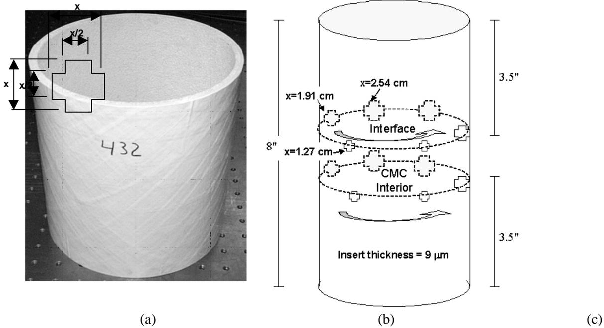
Fig 6. Oxide/oxide delamination test sample. a) photo of cylinder test sample b) schematic diagram showing position of delams, c) size description of intentional delams.
