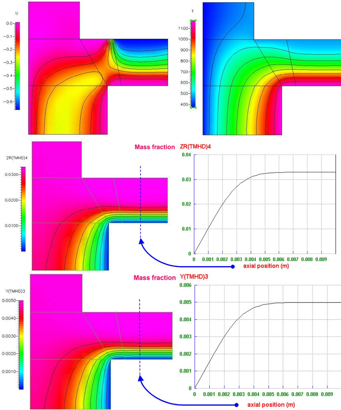
Figure 2. Axial velocity (top left) and temperature (top right) are independent of radial position near the center of the reactor. Depletion of  $Zr(tmhd)_4$  (middle) and  $Yr(tmhd)_3$  (bottom) at substrate indicates that deposition rate is limited by diffusion across a mass transfer boundary of approximately 3.5 mm width.
