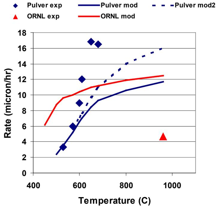
Figure 4. Surface reaction rate is based on Pulver (reference 3) low temperature results. At high temperature, deposition is limited by mass transport.
