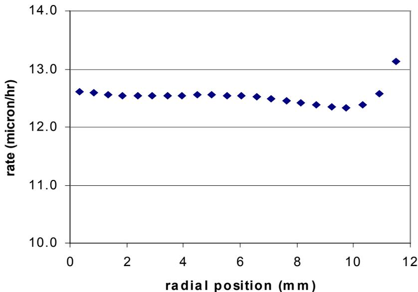
Figure 3. Model predicts uniform deposition rate ( $\pm 0.7\%$ ) within 1.0 cm of the center of the substrate. For these conditions, ORNL observed a deposition rate of 4.7 micron/hr.
